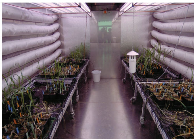
Figure 1. 3 : chambre de culture C (68 tubes fluorescents Osram Fluora 58W)
