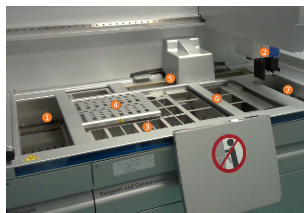
Figure 2. Automate de purification QIASymphony SP.
